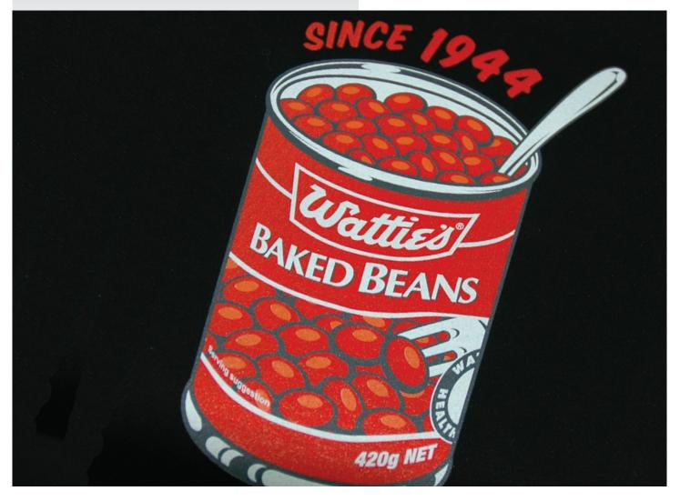
This is the most common type of screen prints. Art is separated into the different colours and a screen is made for each. With a dark shirt a white base print is put down and the colours go on top of this. It is a little more expensive than printing on a white shirt as each colour needs to be cured before the next colour goes on.
