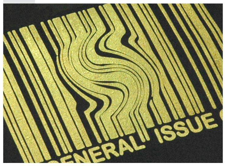
This is a process that gives a mirror like finish to a print or part of a print. We can print up to 2 foil colours in a print. Available in a range of colours.
